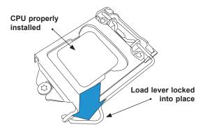
**Note:** You can only install the CPU in one direction. Make sure it is properly inserted into the socket before closing the load plate. If it doesn't close properly, do not force it as it may damage your CPU. Instead, open the load plate again and double-check that the CPU is properly aligned.
