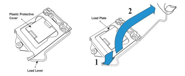
2. Gently lift the load lever to open the load plate. Remove the plastic protective cover. Do not touch the CPU socket contacts.
