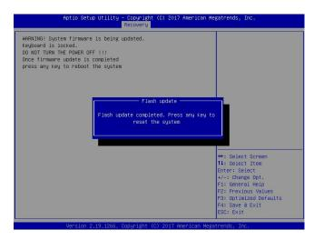
Note: Do not interrupt the BIOS flashing process until it has completed.
