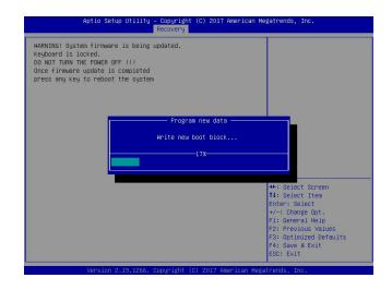
4. When the screen as shown above displays, use the arrow keys to select the item "Proceed with flash update" and press the <Enter> key. You will see the BIOS recovery progress as shown in the screen below:
