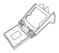
3. Locate the triangle on the CPU and CPU socket, which indicates the location of Pin 1. Holding the CPU by the edges with your thumb and index finger, align the triangle on the CPU with the triangle on the socket. The CPU keys (the semi-circle cutouts) may also be aligned against the socket keys as a guide.
