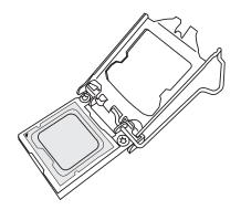
5. Close the load plate, then gently push down the load lever into its locking position.
