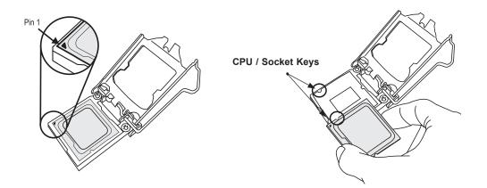
4. Carefully lower the CPU straight down into the socket. Do not drop the CPU on the socket, or move it horizontally or vertically to avoid damaging the CPU or socket. Inspect the four corners of the CPU to make sure that the CPU is properly installed.
